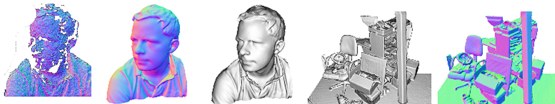
Figure 1: Example output from our system, generated in real-time with a handheld Kinect depth camera and no other sensing infrastructure. Normal maps (colour) and Phong-shaded renderings (greyscale) from our dense reconstruction system are shown. On the left for comparison is an example of the live, incomplete, and noisy data from the Kinect sensor (used as input to our system).
