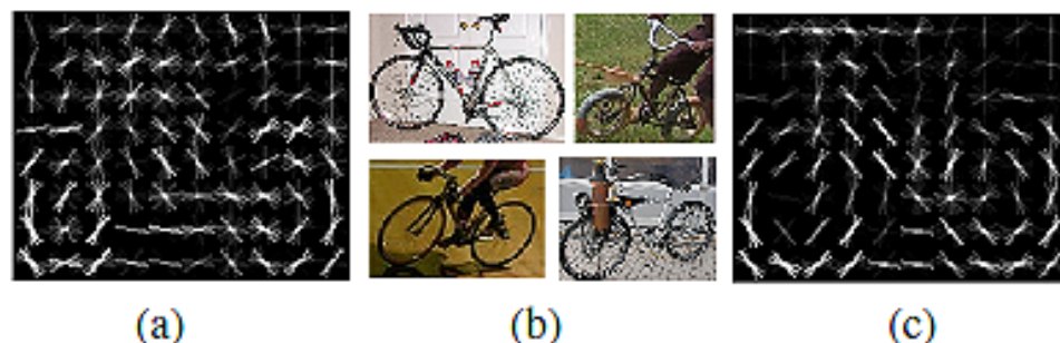
Figure 1. The benefit of transfer learning. The learnt HOG detector template for a motorbike (a) is used as the source for learning a bicycle template together with the samples shown in (b). The resulting learnt bicycle HOG detector template (c) clearly has the shape of a bicycle. Note, here and in the rest of the paper we only visualize the positive components of the HOG vector.
